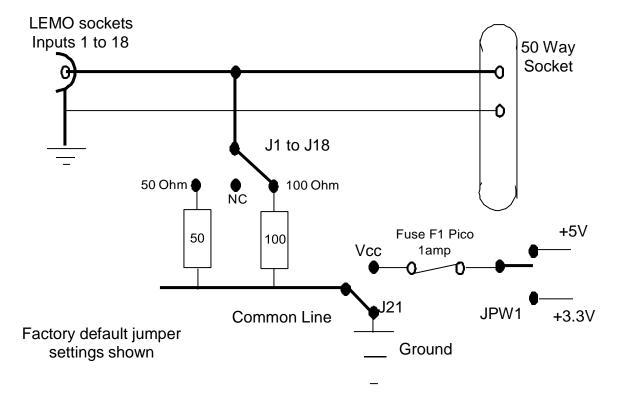
Each of the 16 signal inputs can be set to have no termination, 100 ohms termination or 50 ohms termination by selecting the positions of jumpers J1 to J16 in one of three positions. If 50 or 100ohms are selected they are connected to a common line that can be connected to ground, or by connecting an external power supply, to +5 Volts or +3.3Volts.
